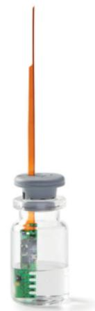
A single-use probe, containing 5 independent temperature sensors including wireless communication which is placed within the vial.
