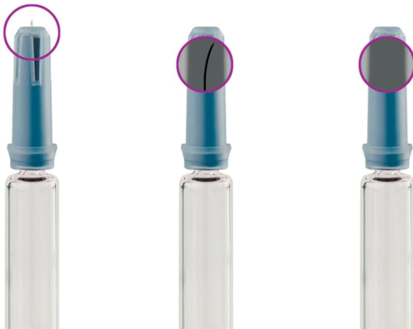
Figure 2: The pulsed X-ray technology makes visible what is difficult or impossible to see visually: pre-fillable syringes with punctured needle shields, bent or missing needles.
